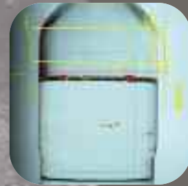
Level control (back light)
